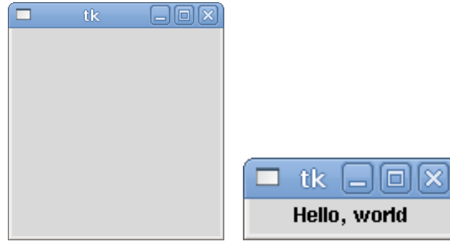
Figure 2.3: Outputs of (a)tkmain.py (b)tklabel.py
