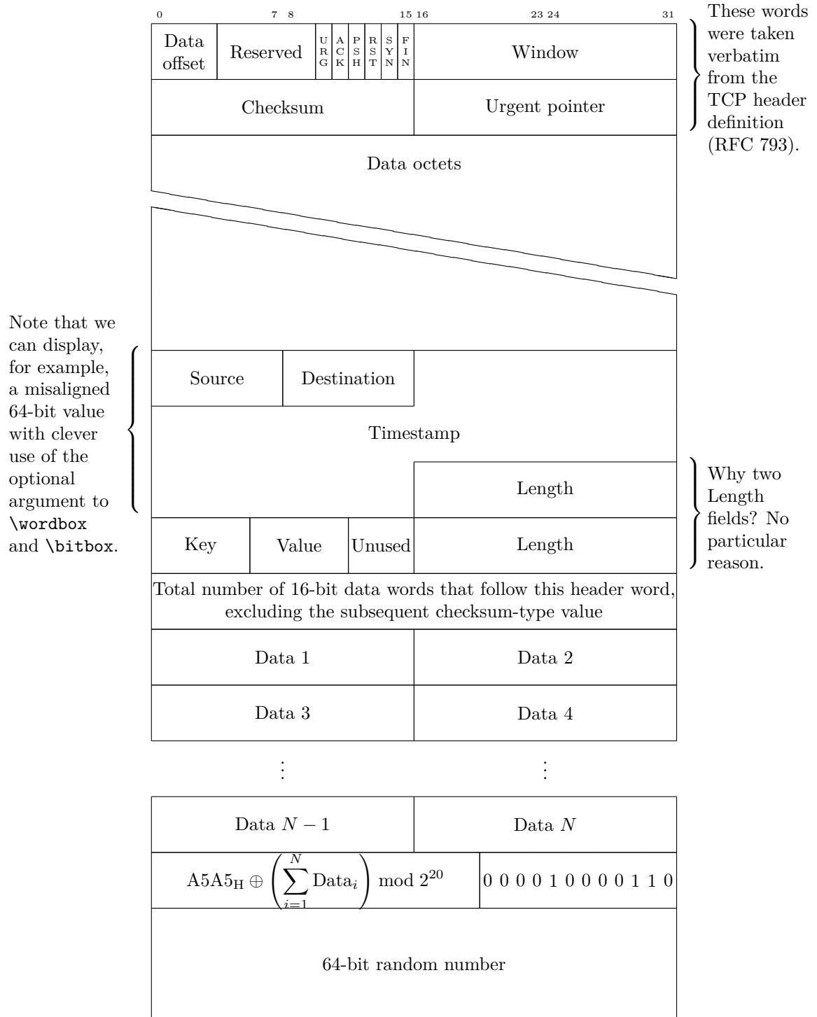
Figure 3: Complex protocol diagram drawn with the `bytfield` package
